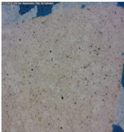
Typical ceramic coating shows pinholes and cracks
